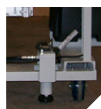
Auto-lock System All auto-lock systems use cylinders to lift the unit in use, so the unit does not move during operation.
