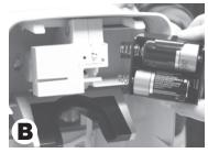
**B.** Insert Battery Pack into Electronic Module with contacts touching (this will activate the unit).
